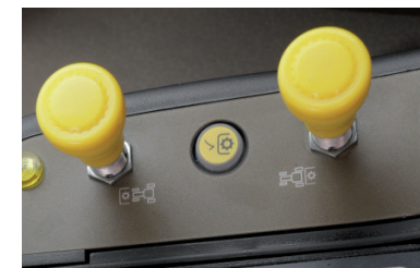
Electro-hydraulic activation of the rear and front PTO.
